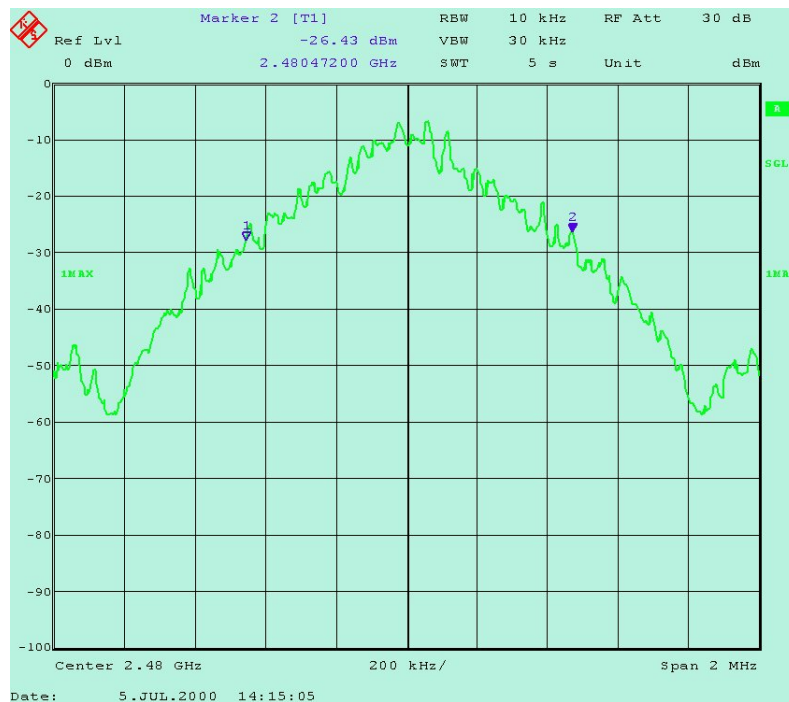
Fig. 13 TX output spectrum – 20 dB bandwidth: results displayed by analyzer
